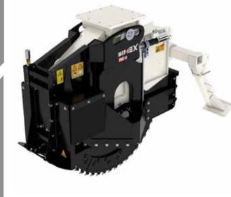
Intended for excavator boom mounting, they are specially indicated for cutting and narrow trenching for fiber optics installation on hard and compact surfaces: asphalt, concrete and rock. Slides parallel to the ground. Constant trenching depth. Mechanical or hydraulic adjustment of trench depth. Disk with removable, interchangeable segments allows quick variation of the trench width while maintaining the same base wheel. (RWE 50).
